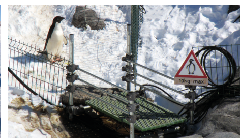
Gateway identification / automatic weighing
